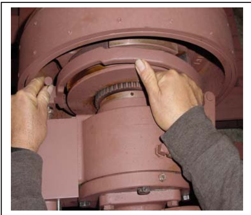
REINSTALL THE AIR CYLINDER AND WHILE PUSHING ON THE CLUTCH YOKE INSURE THAT THE PIN DROPS IN FREELY
