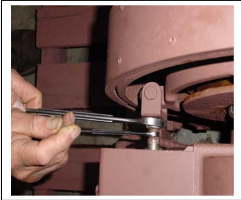
HOLDING THE CYLINDER ROD LOOSEN THE JAM NUT
