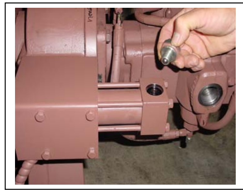
INSPECT ROLLER BALL ON BOTTOM OF SWITCH
